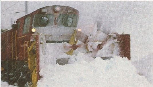
Through the snow by train: the high-performance, rotary snow ploughs blast 19 tons of snow from the tracks – per minute!
