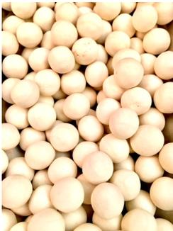
The unique latent heat storage capabilities of the Zeolite pellets allow them to release heat by just adding water. They can be recharged with solar vacuum tube heat.
