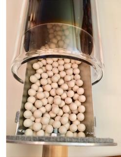
The solar thermal vacuum tube can efficiently heat to recharge Zeolite pellets. Without a reflector it can heat up to 212 F or 100 C. With reflectors up to 400 F or 204 C.
